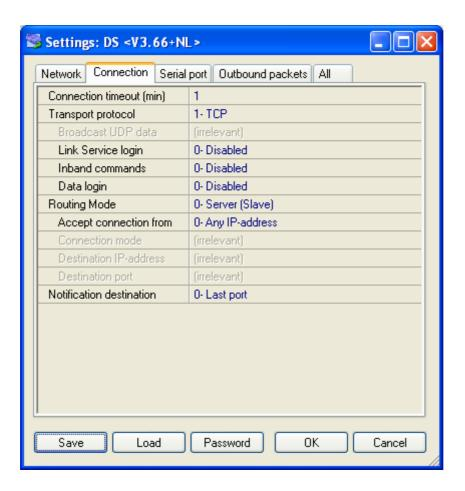
In the connection Tab, it's important to set the Transport protocol to TCP. Connection timeout is up to you, depending on your application (a zero will disable timeout). Routing Mode should be "0-Server (Slave)". Unless you want to accept connections from only a single IP address, leave the 'Accept connection from' box to 'Any IP-address'.
